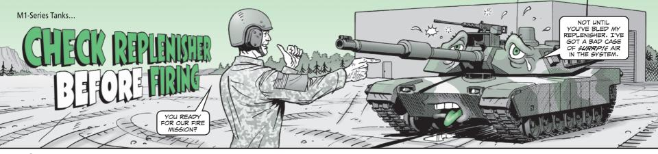
Grewmen, your M1's main gun could recoil uncontrollably the next time it's fired if the recoil system has too little fluid or too much air. When either happens, the cannon can shear its retaining bolts and slam into the ammo compartment—definitely not something you want happening to you or anyone else in the turret!
