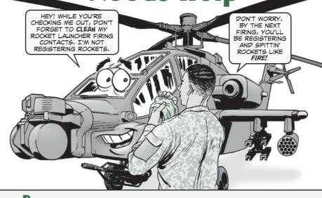
Repairers, when you load rockets into your AH-64's M261 rocket launcher, you know something isn't right if the rockets don't register.
